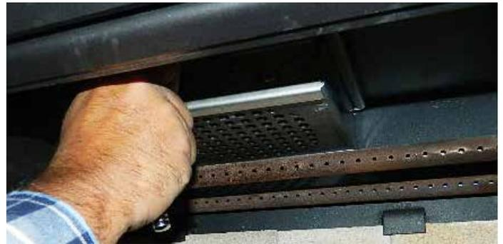
9. Loosen bolts on catalyst retainer then, slide the catalyst retainer to the right to remove.
