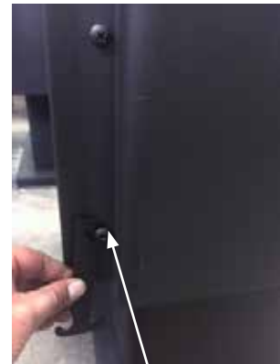
Loosen screw and insert storage bracket.
