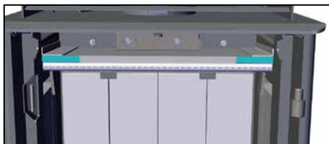
Baffle brackets and cover plates in final position
