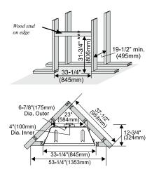
\*\*\* NOTE: If using the optional Vignette finishing trim, this can be installed as a 3-sided or 4 sided finish trim. If choosing to use this as a 4 sided finish trim the framing would need to be increased in height by 1-1/4" inches minimum in order for this to fit. This must be to the finished floor. (Example: 34 3/4" framing height + 1-1/4" to bottom of 4-sided finishing trim +1/2 thick finished floor = 36 1/2" total framing height
