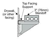
Frame in the enclosure for the unit with framing material - see next page for dimensions.
