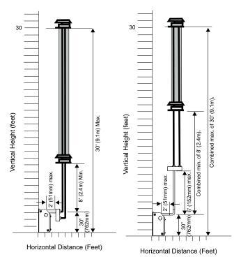
The shaded area in the diagrams show the allowable vertical terminations.
