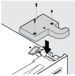
2. After the hinge covers are removed, disconnect any harnesses between the cabinet and doors by grasping both sides of the connector firmly, depress the latch and pull apart.
