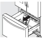
Push inward slightly on the basket tabs to release the upper basket from the slide assemblies (1 per side, in front).
