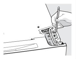
4. Remove bulkhead cover at rear of unit to access water tubing. Disconnect the water tube at the push-lock connection on the rear of the unit below the bulkhead. The dispenser line is connected to the yellow water line coming from the main water valve.
