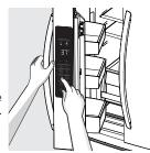
Continue dispensing water for about four minutes to flush the system and plumbing connections of any impurities (stopping to empty the glass as necessary).
