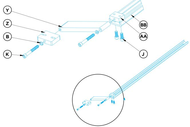
Vertical speaker mounting rails, with hinges, have been preassembled. Image below shows preassembled parts and hardware, in exploded view.
