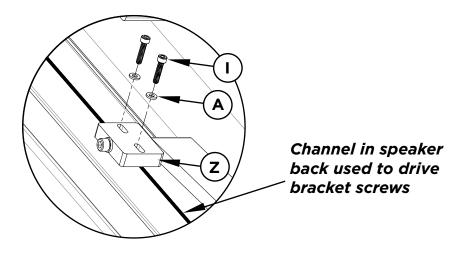
7. Ensure speakers are properly aligned with TV before tightening all screws and threaded rods with nuts (G) if applicable, only when using threaded rod (T). Now, tighten screws securely.
