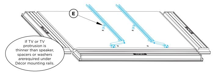
3. Position the assembled VERTICAL speaker rail assemblies on top of the HORIZONTAL speaker rails. Align the rails so holes match up.
