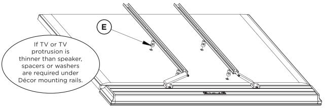
4. Take additional TV rails included in separately purchased TV wall Mount Kit and place onto back of TV overtop of attached speaker rail assemblies.
