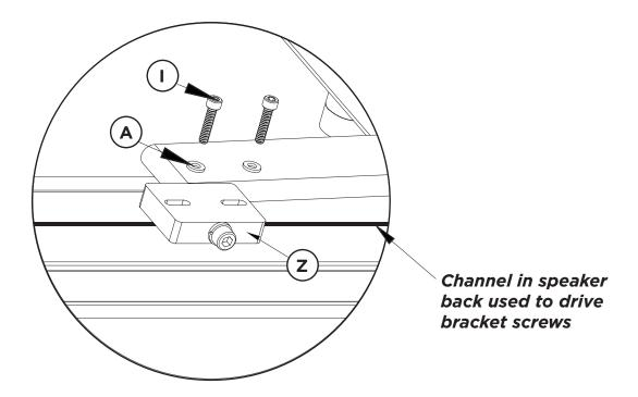
7. Ensure speaker is properly aligned with TV before tightening all screws and threaded rods with nuts (F) if applicable, only when using threaded rods (T).
