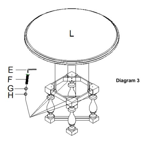
4. Sit table top (L) on base frame. Align holes and use flat washers (H), lock washers (G) and bolts (F), tighten with allen wrench (E). (See Diagram 3)
