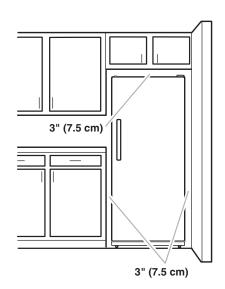
**IMPORTANT:** Do not install the freezer near an oven, radiator, or other heat source, nor in a location where the temperature will fall below 40°F (5°C).
