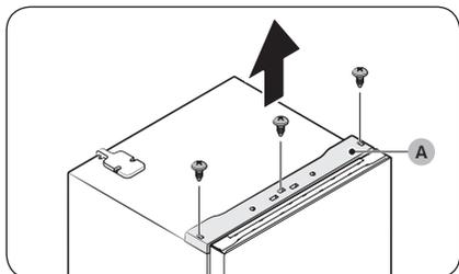
1. Use a Phillips screwdriver to remove the screws on the **top table (A)**. Then, gently pull out the **top table (A)**.
