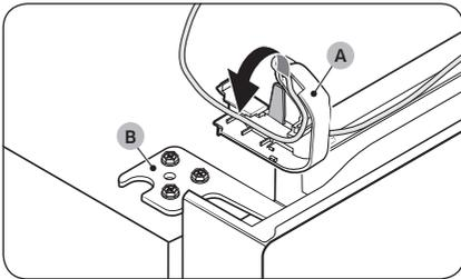
34. Arrange the door wire in the hinge cover (A) before placing the hinge cover (A) onto the top hinge (B).
