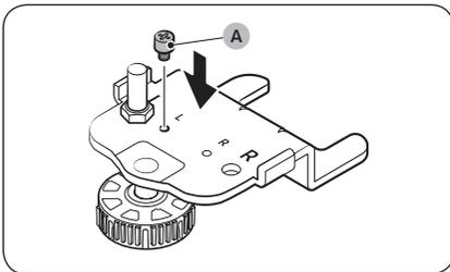
10. Insert the **hinge bolt (A)** into the hole next to the hinge shaft as shown in the figure, and then tighten it until it is securely in place.
