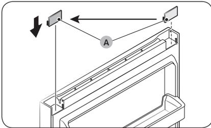
22. Remove the cap spacer (A), and then reinsert it on the opposite side.
