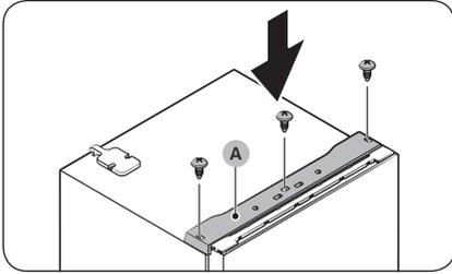
38. Insert the **top table (A)**, and then fix it firmly to the refrigerator using the screws (x3).
