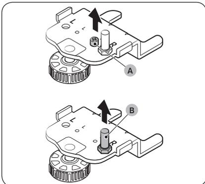
8. Use a screwdriver to remove the **hinge bolt (A)**. Then, use a spanner to remove the **hinge shaft (B)**.
