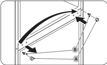
25. Use the flat-head screwdriver to remove the **flange-screw cap (A)** to reveal the **flange screw (B)**. Use a Phillips screwdriver to remove the **flange screw (B)**, and then tighten it on the opposite side. Finally, close the **flange-screw cap (A)** on the opposite side.
