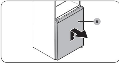
6. Gently lift the **fridge door (A)** to remove it from the bottom hinge.
