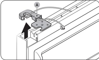
17. Remove the top hinge (A) with its cover.
