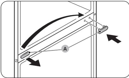
24. Use a flat-head screwdriver to remove the **middle-hinge screw cap (A)**, and then reinsert it on the opposite side.
