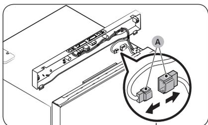
2. Decouple the **wire connectors (A)**.
