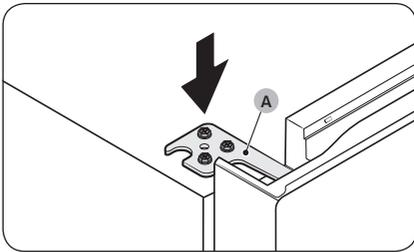
32. Insert and fasten the top hinge (A) on the opposite side.
