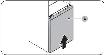
29. Align the middle hinge shaft to the hinge grommet on the top of the **fridge door (A)**. Then, lift the door and hold it so the shaft is inserted into the grommet.
