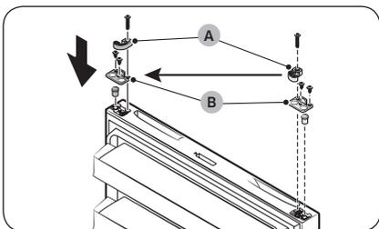
15. Remove the **auto closer (A)** and the **stopper (B)** from the bottom of the fridge/freezer doors. Then, reinsert them on the opposite side of the fridge/freezer doors as shown in the figure.
