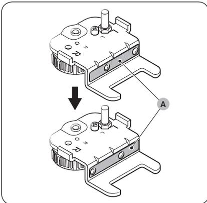
11. Flip the **hinge shim (A)** 180 degrees as shown in the figure.
