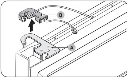
18. Separate the top hinge (A) and the hinge cover (B).
