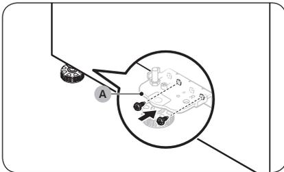
30. While one person holding the fridge door, fasten the **bottom hinge (A)**.
