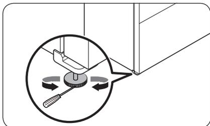
To level the refrigerator, use a flat-head screwdriver to turn the leveling leg clockwise or counterclockwise. Turn the leveling leg clockwise to raise, and counterclockwise to lower the height.
