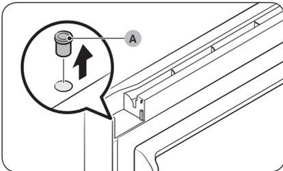
20. Use a flat-head screwdriver to remove the hinge grommet (A).
