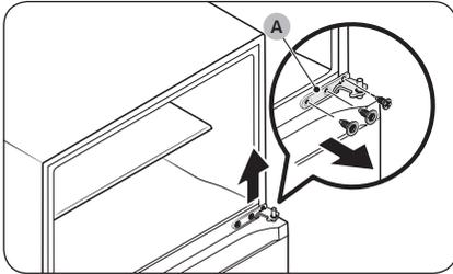
5. Use a screwdriver to remove the screws and then detach the **middle hinge (A)**.
