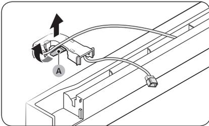
19. Take out the wires from the hinge cover (A).
