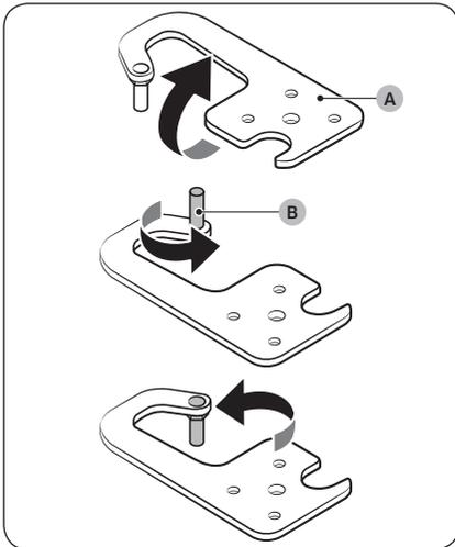
23. Flip the top hinge (A) 180 degrees. Remove the hinge shaft (B), and then reattach it facing down.
