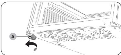
13. Remove the **leveling leg (A)** attached to the left side of the main unit.
