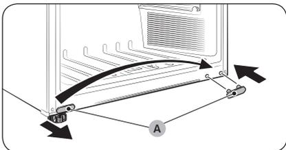
12. Use a flat-head screwdriver to remove the **bottom-hinge screw cap (A)**, and then reinsert it on the opposite side.
