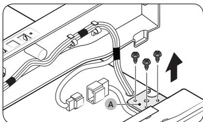
3. Remove the screws fastening the **top hinge (A)**.
