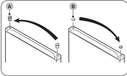
28. Use the flat-head screwdriver to remove both the **hinge grommet (A)** on one side and the **hinge-hole cap (B)** on the other side. Reinsert them on their respective opposite side.
