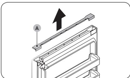
16. Pull up to remove the **bar cover (A)** on the top of the freezer door.
