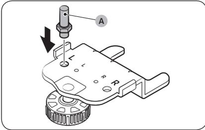
9. Insert the **hinge shaft (A)** into the leftmost hole on the bottom hinge plate as shown in the figure, and then tighten it until it is securely in place.
