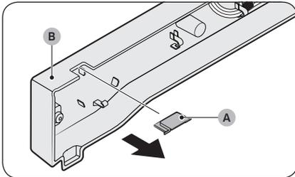
36. Remove the hinge hole cap (A) from the top table (B), and then reinsert it on the opposite side.
