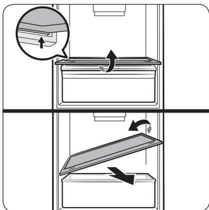
2. Hold the vegetable shelf with both hands and lift it to release it from the rear hook. Then, tilt it on one side and pull it out.
