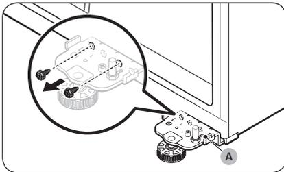
7. Use a screwdriver to remove the screws fastening the **bottom hinge (A)**.
