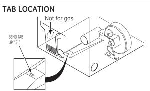
Through the rear opening, locate the tab in the middle of the appliance base. Lift the tab to about 45°, using a flat-blade screwdriver.
