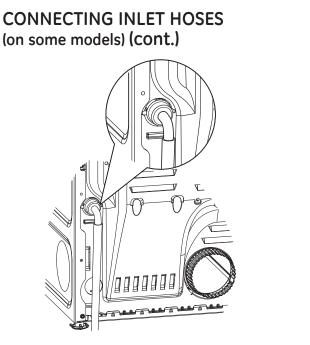
7. Using pliers, tighten all the couplings with an additional two-thirds turn.
