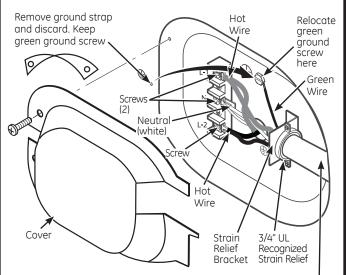
4 #10 AWG minimum copper conductors or 120/240V 30A power supply cord kit marked for use with dryers and provided with closed loop or spade terminals with upturned ends (not supplied).
