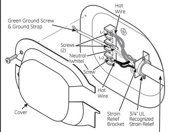
3 #10 AWG minimum copper conductors or 120/240V 30A power supply cord kit marked for use with dryers and provided with closed loop or spade terminals with upturned ends (not supplied).
