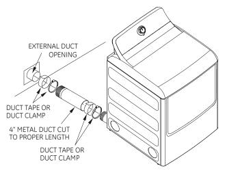
**NOTE:** We strongly recommend using rigid metal exhaust duct. However, if flexible ducting is used it must be UL-Listed metal, not plastic.
