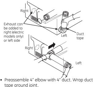
• Insert duct assembly, elbow first, through the side opening and connect the elbow to the dryer internal duct.
