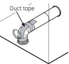
Internal duct joints must be secured with tape; otherwise, they may separate and cause a safety hazard.
