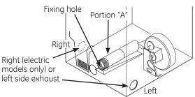
Reconnect the cut portion (A) of the duct to the blower housing. Make sure that the shortened duct is aligned with the tab in the base. Use the screw saved previously to secure the duct in place through the tab on the appliance base.
