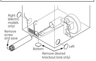
Detach and remove the right (electric models only), left or bottom knockout as desired. Remove the screw inside the dryer exhaust duct and save. Pull the duct out of the dryer.
