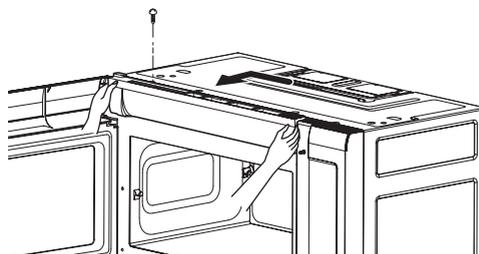
4. Remove the cover screw slide the cover to left and then lift up the bulb holder.
