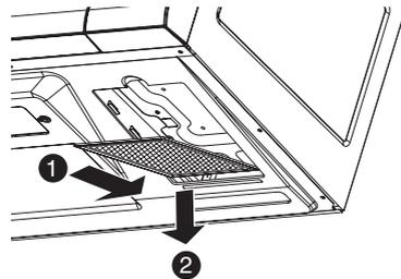
2. Soak grease filters in hot water and a mild detergent. Rinse well and shake to dry. **Do not use ammonia or place them in a dishwasher. The aluminum will darken.**
