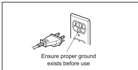
For a permanently connected appliance: This appliance must be connected to a grounded, metallic, permanent wiring system, or an equipment grounding conductor should be run with the circuit conductors and connected to the equipment grounding terminal or lead on the appliance.
