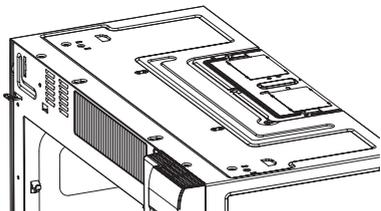
6. Slide in vent grille and replace the mounting screw. Turn the power back on at the main power supply and set the clock.
