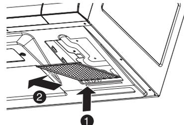
**NOTE:** Do not operate the hood without the filters in place.
