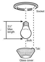
**ACAUTION** Before replacing your oven light bulb, disconnect the electrical power to the range at the main fuse or circuit breaker panel. Be sure to let the light cover and bulb cool completely.
