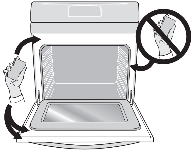
Figure 23: Clean around the oven door gasket
