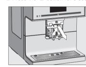
■ Pull the stainless steel cover off and ther pull the dispensing unit off.
