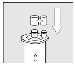
Seal the descaling cartridge with the cap.
