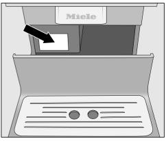
The password of your coffee machine is the serial number located on the data plate.
