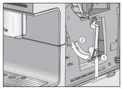
Press and hold the button under the brew unit handle ① and, while doing so, turn the handle to the left ②. Carefully pull the brew unit out of the coffee machine.
