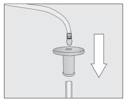
First attach the connecting piece to the long stainless steel tube and then connect the milk pipe to the connecting piece.
