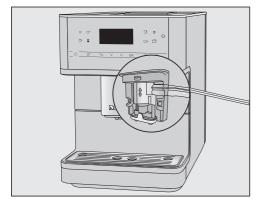
**Tip:** The "seam" on the milk pipework and on the main dispenser makes it easier to assemble.
