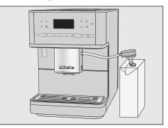
Open the milk carton and dip the milk siphon into the milk. Place the milk carton to the right next to the coffee machine.  Connect the milk pipework to the aperture in the main dispenser.
