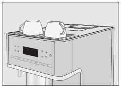
Arrange the cups or glasses on the cup heating surface on the top of the coffee system.
