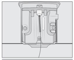
Push the cleaning brush a maximum of 1/2" (1 cm) into the steam jet.
