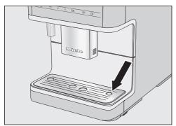
Refit the drip tray cover. Make sure that the drip tray cover is correctly installed (see illustration).
