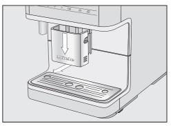
Push the main dispenser down completely and remove the stainless steel cover by pulling it off toward you.
