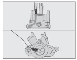
Angle the cleaning brush slightly and clean both spouts from above and below.
