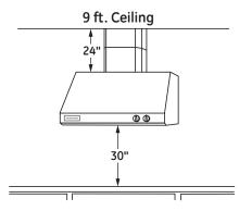
**9 ft. ceilings:** When the hood is installed 30" above the cooking surface, order two 12" duct cover accessories.
