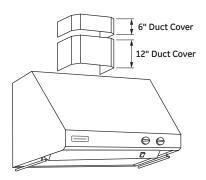
Decorative duct covers are available in 6" and 12" heights. Duct covers may be stacked, in various combinations, to conceal the ductwork running from the top of the hood to the ceiling.
