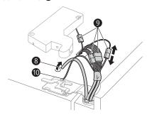
Rotate the hinge lever **10** counterclockwise. Lift the top hinge @ free of the hinge lever latch **B**.
