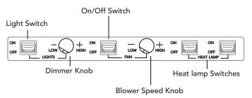
Fan On/Off switch—Starts and stops the blower. When turned on the blower will operate at the previous setting of the speed control.
