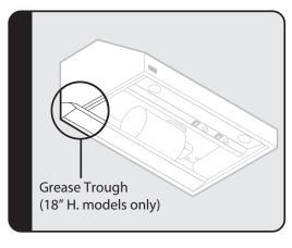
When cleaning filters in 18"H. hoods, always remove the grease trough and clean by soaking in a sink with hot soapy water.
