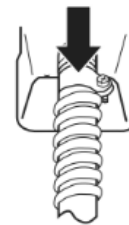
A. Removable retaining nut B. Conduit
