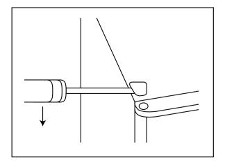
2.Unscrew the top hinge with a Philips screwdriver.
