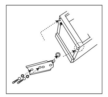
9.Stand up the refrigerator upright and put the door on the bottom hinge. Make sure the bottom hinge core is inserted in the door hole. Then move the hinge hole "plug" of bottom door left side to right side.
