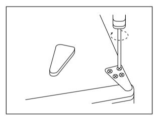
4.Move the "plug" cover from the left side to the right side then lift the upper door and place it on a padded surface to prevent it from scratching.
