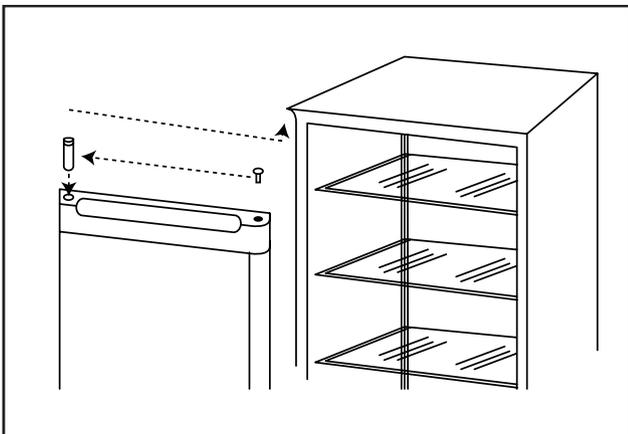
10. Install upper hinge to connect the top portion of door to the unit. Clap in the hinge cover and hold cover on top of the unit.
