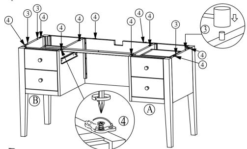
5. Insert (3/4") flat head wood screws (10 PCS) through metal figure 8 bracket to connect desk top (E) and pedestals (A) and (B). Use (1-1/4") flat head wood screws (1 PC) to connect cross bar (D) to desk top (E).
