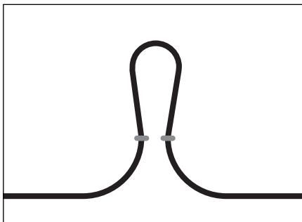
2. Recommended: Use a wire tie (not included) to keep the wire loop intact and act as a strain relief.
