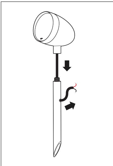
2. To attach the speaker to the ground stake, hand thread the speaker to the ground stake.
