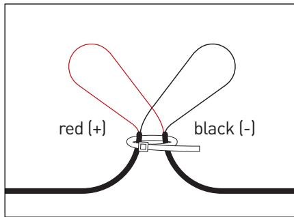
4. Cut the red (+) and black (-) wires with cable strippers and strip off 1 inch (25.4mm) of insulation to expose the bare wire conductor.
