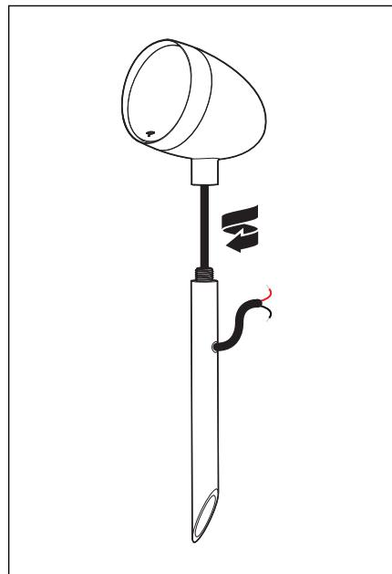
3. By hand, push the speaker assembly into the ground.
