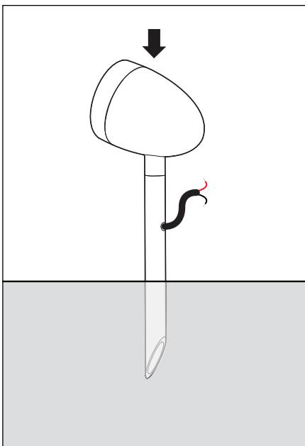
4. The speaker is now installed. The next step is wiring, go to the next page for instructions.
