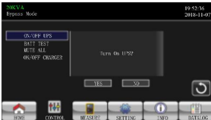
TURN ON UPS
