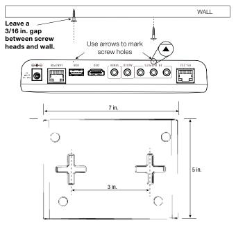
*Structured Wiring Cabinet Mounting:* Using the optional Structured Wiring Cabinet Mount, the EL-SC-100 can be mounted in a structured wiring cabinet.
