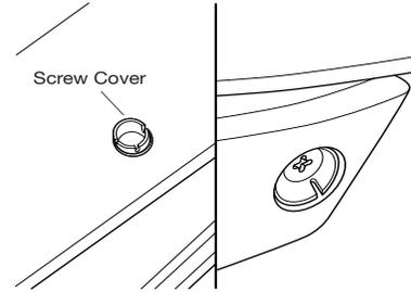
6. Install the 4 screw covers with bump going into the recess.
