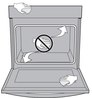
Figure 11: Do not clean oven door gasket
