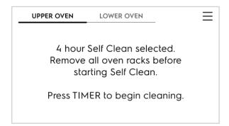
When the oven is set to run a self-clean cycle, the motor door lock will begin locking the oven door. Do not open the oven door while the lock motor is running or when any locking indicators or displays are showing. The oven door is completely locked in about 15 seconds. Once the oven door has locked, CLEAN will appear in the display indicating self clean has started.
