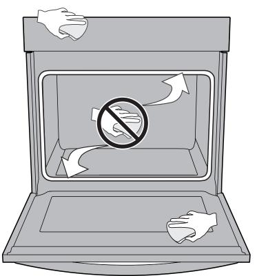
Figure 6: Do not clean oven door gasket
