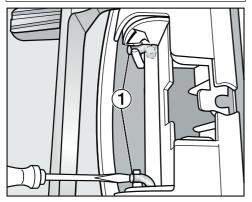
■ Insert the end of the screwdriver blade under rod ① and rotate it so it is in an upright position. Do the same to the other rod.
