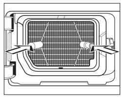
■ Push the plinth filter in completely.
