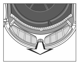
Hold the dial and pull the lint filter forward to remove it.
