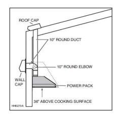
The custom hood must be constructed to fit the size and shape of the liner (power pack). See chart and illustration below for details.
