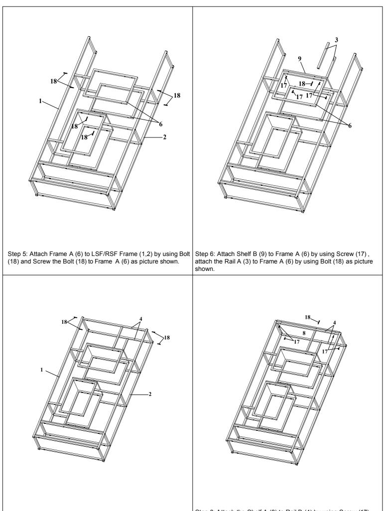
Step 7: Attach the Rail B (4) to LSF/RSF Frame (1,2) using Bolt (18) as picture shown.
