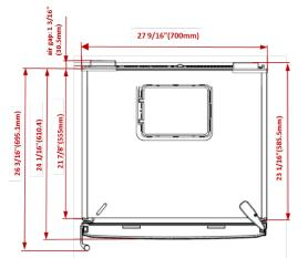
**Required minimum air gap clearances:** 1 ½" top, 1/8" sides, 1 3/16" back
