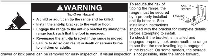
drawer or kick panel can be removed for easy inspection. If visual inspection is not possible, slide the range forward, confirm the anti-tip bracket is securely attached to the floor or wall, and slide the range back so the rear leveling leg is under the anti-tip bracket.
