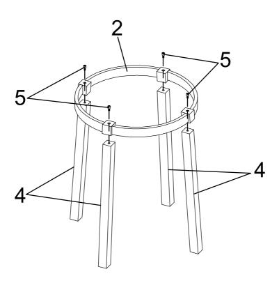
Step 1: Attach Table Leg (4) to Top Frame (2) using Hex Cap Head Bolt (5).
