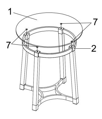
Step 3: 1.Insert Suction Cup (7) into Top Frame(2). 2.Place the Glass Top (1) onto the Suction Cup (7).
