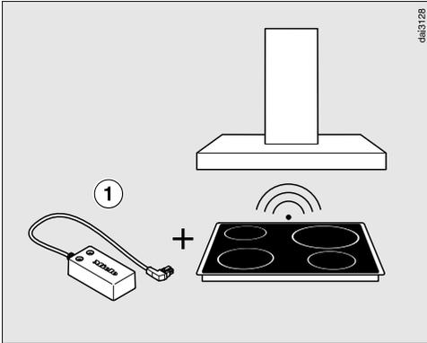
To enable the communication function, the cooktop must be equipped with the corresponding Con@ctivity 2.0 stick ①.
