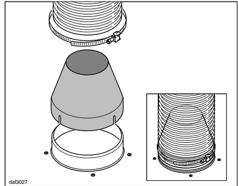
If you would like to reduce the environmental impact of your ventilation system by limiting the CFM output the Reducing Collar can be installed. It reduces the air flow to less than 400 CFM. Check local building codes for max. CFM requirements.
