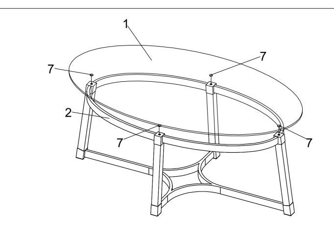
Step 3: 1.Insert Suction Cup (7) into Top Frame(2). 2.Place the Glass Top (1) onto the Suction Cup (7).
