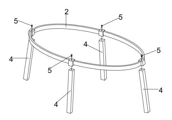
Step 1: Attach Table Leg (4) to Top Frame (2) using Hex Cap Head Bolt (5).
