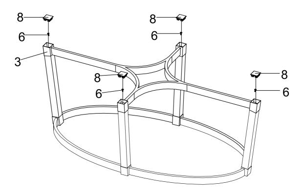
Step 2: 1. Attach Bottom Frame(3) to the assemble in Step 1 using Bolt (6). 2. Insert Cap (8) into Bottom Frame (3).
