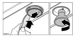
Insert the lever supplied into the gap between the bulb and the bulb holder.
