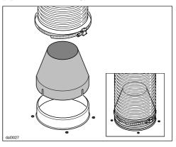
If you would like to reduce the environmental impact of your ventilation system by limiting the CFM output the Reducing Collar can be installed. It reduces the air flow to less than 400 CFM. Check local building codes for max. CFM requirements.
