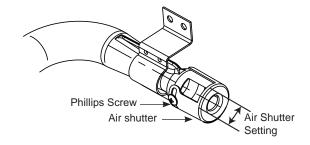
With a Phillips head screwdriver, loosen the screws securing the air shutters on the burners and adjust the air shutters according to chart.
