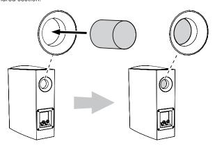
CAUTION: Be careful not to insert the port plug so far into the port tube that it falls inside of the speaker.
