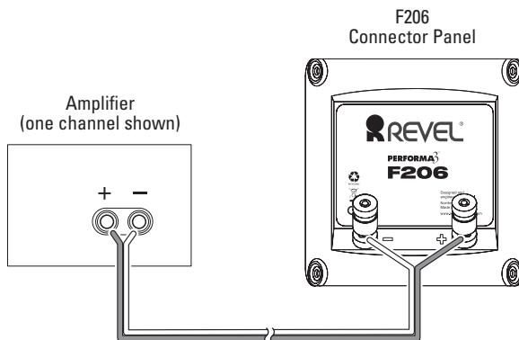
Connect both loudspeakers using the same method, using speaker cables of the same length for each speaker.
