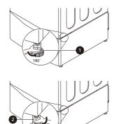
7 Turn all 4 leveling feet 1 in one direction to raise the pedestal or the other direction to lower it. Then tighten the locknuts 2.
