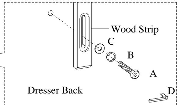
**STEP 2:** Attach the wood strip to the mirror by using 4 bolts(A), lock washers(B), and flat washers(C). Tighten all bolts on dresser and mirror with Allen wrench.
