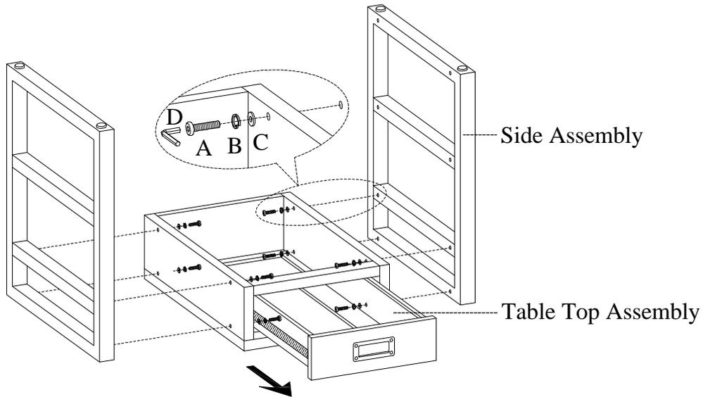
**STEP 3:** Attach the shelves to the side assemblies by using 8 bolts (A), lock washers(B) and flat washers(C). Use the Allen wrench provided to tighten all the bolts.
