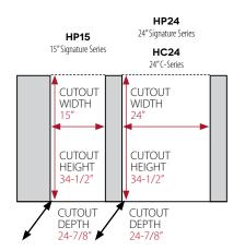
\* For all HP, HC, and HA models. To achieve 24" installation depth, install electrical connection in adjecent cabinetry. See spec sheets and installation instructions for install instructions.
