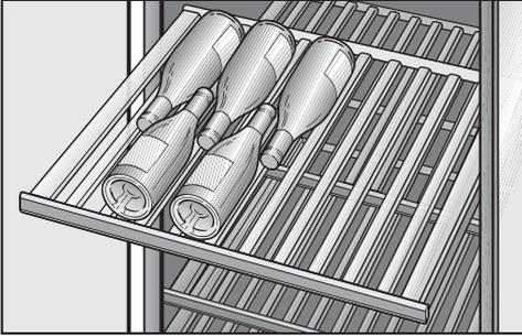
The wooden shelves are mounted on telescopic runners which can be pulled out to make it easier to store and remove bottles.
