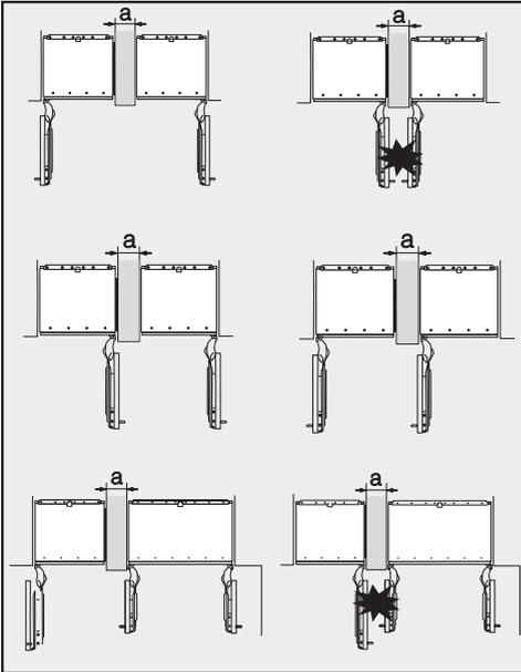
If the partition wall **a** is **narrower than 6 5/16" (160 mm)**, you will need the side panel heater from the side-by-side installation kit to prevent condensation from forming and any resulting damage.
