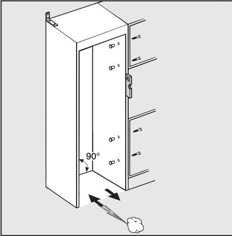
The installation niche must be carefully aligned using a bubble level before installing the wine conditioning unit. The niche corners must be at 90° angles to each other, otherwise the cabinet front will not sit straight on all 4 corners of the installation niche.
