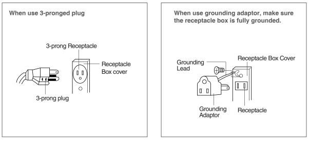
"THE CANADIAN ELECTRICAL CODE DOES NOT ALLOW THE USE OF THE GROUNDING ADAPTOR"
