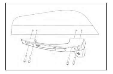
2. Insert the one side of handle cover into the handle pedestal.
