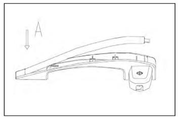
3. Insert the other side of handle cover into the handle pedestal.
