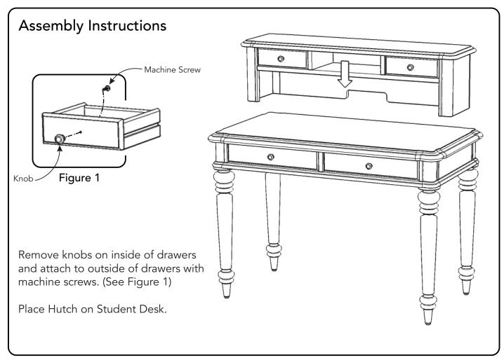
Tool(s) required for assembly: Phillips screwdriver
