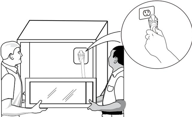
3. Slide the microwave oven back and into place.
